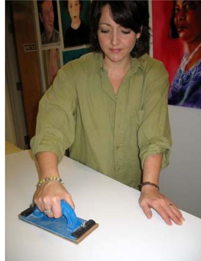
2. The panels are lightly sanded with 100-grit sandpaper - just enough to dull the sheen and provide a tooth for the primer. Avoid over-sanding, as this will expose the bare aluminum.
